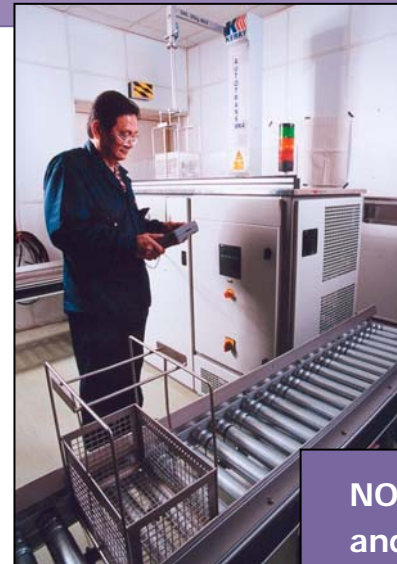
Kerry Microsolve 350 co-solvent system with solvent usage monitoring and auto top-up device
